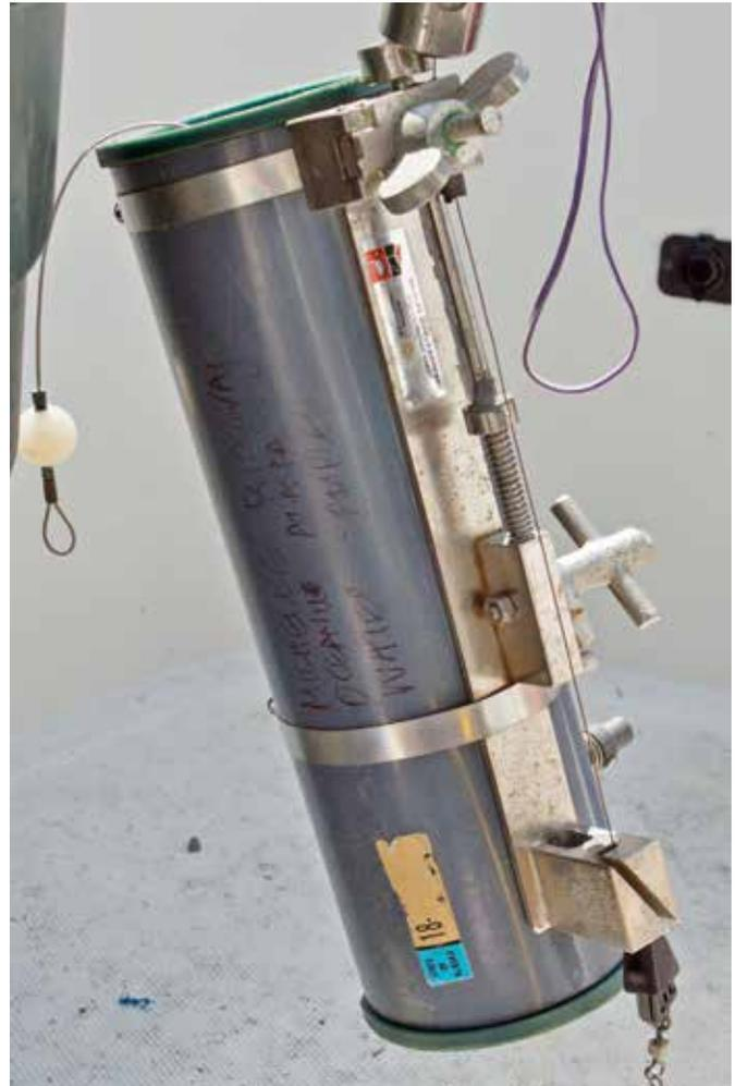
When Niskin water sampling bottle reaches desired depth with both ends open, weighted messenger is sent down wire to trigger closure. The bottle is retrieved having captured the sample.
